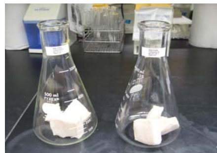
Figure 4: Cut foam in Erlenmeyer flasks for batch process.
